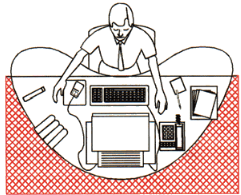
Figure 1: Alignment and Desk Set-up
